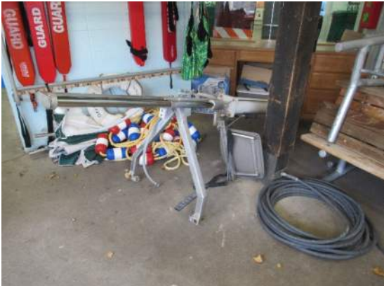
ADA chairlift stored in bathhouse
